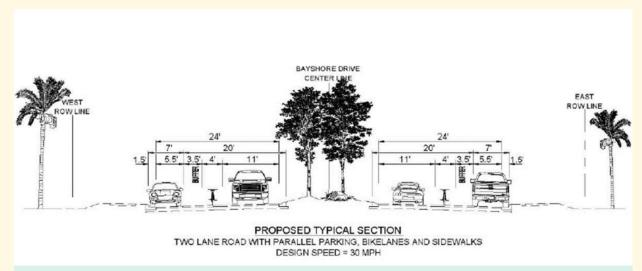
Potential cross section for Bayshore Dr road diet, as proposed in Trebilcock's 2017 Parking Needs Analysis. Existing cross section is four-lane road with bike lanes and sidewalks
