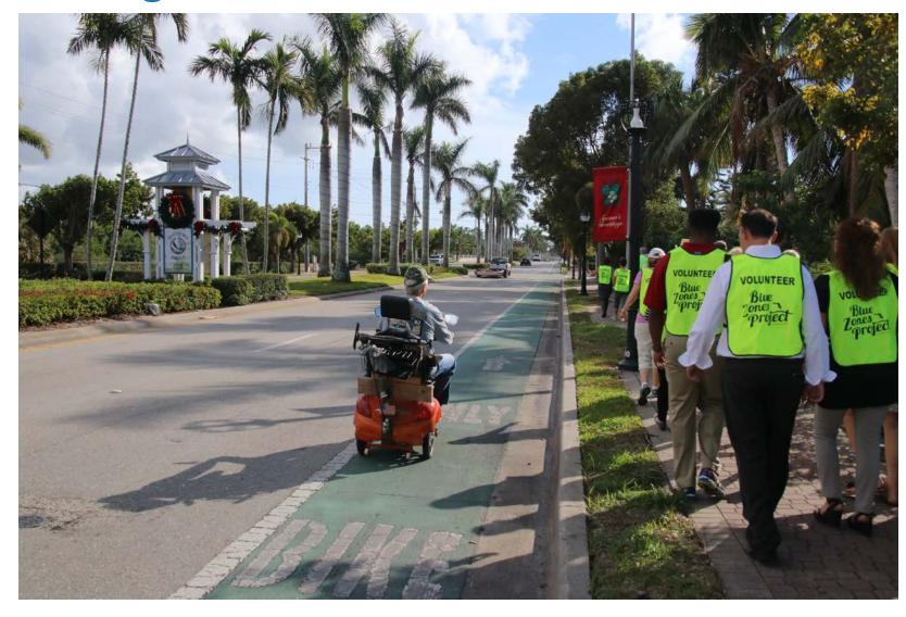
Bayshore Drive uses innovative colorized bike lanes. This conversion of Bayshore, adding the median, tightening the lanes to 10 feet, creating the bike lanes, in 2012, has improved walking and bicycling conditions.
